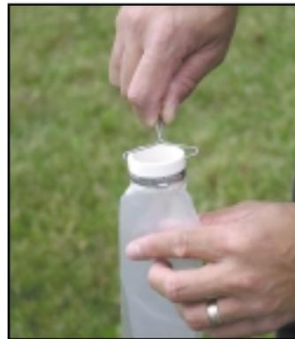
**4** Attach the large clip by inserting the prongs into the holes at the top of the sampler.
