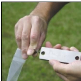
**3** Attach the reusable weight to the clip at the bottom of the sampler.
