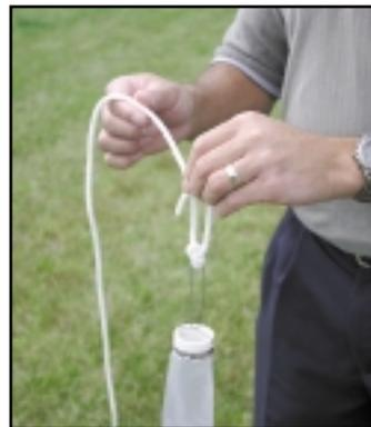
**5** Attach the suspension line to the upper clip. Tie securely.
