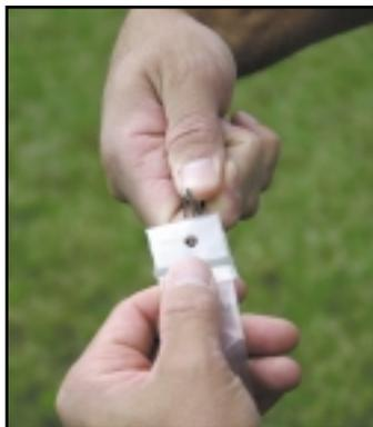
**1** Remove sleeve and the 2 clips from package and unroll the sampler. Attach the small clip by inserting the prongs into the hole at the bottom of the sampler.
