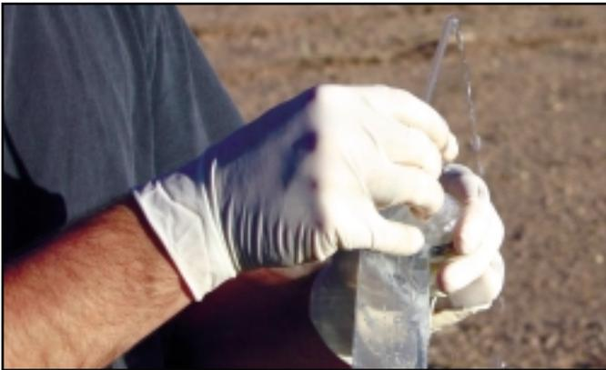
Then, push the pointed discharge tube through the polyethylene sleeve at the base of the top ring. (Photo 2, middle left)
