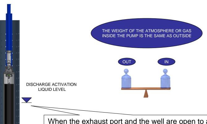
When the exhaust port and the well are open to atmosphere or when the exhaust line is inside the well the liquid level inside the pump to start the discharge cycle is as shown. The gas pressure inside the pump and outside the pump are the same. Only the higher liquid level outside the pump will cause it to fill to the cycle activation level
