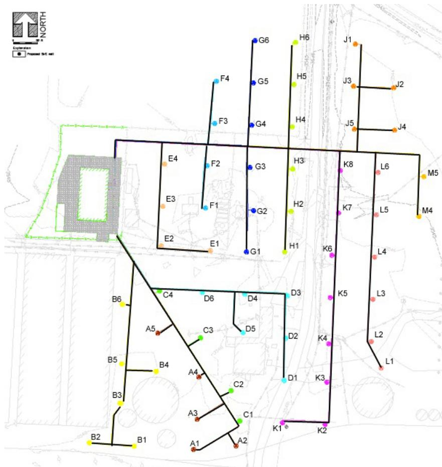
Site Plan showing the soil vapor and groundwater extraction well network and treatment systems location.
