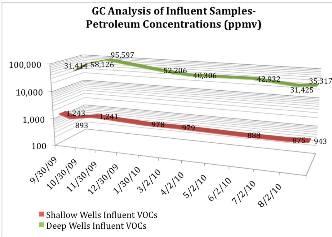
Graph illustrating the influent vapor concentrations in log scale vs date of sampling for the three treatment processes at the site.
