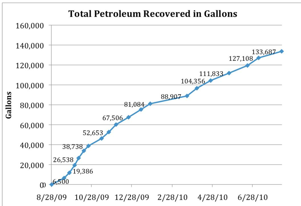
Graph illustrating cumulative gallons of recovered hydrocarbons from the vapor recovery systems at the site. Recovery of hydrocarbons appears to be fairly constant.
